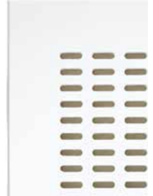
Tangent, 4 x 14 mm, 10/20 mm c/c Perforation: 21.3%
