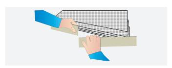
• Remove the cardboard liner around the ceiling tiles.
