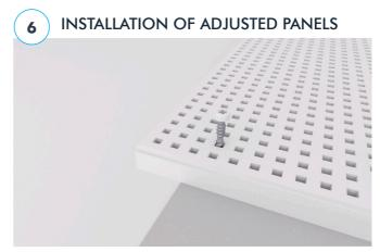
• Place the screws in 4<sup>th</sup> or 5<sup>th</sup> perforation row of the adjusted panel for easier screw-fixing.
