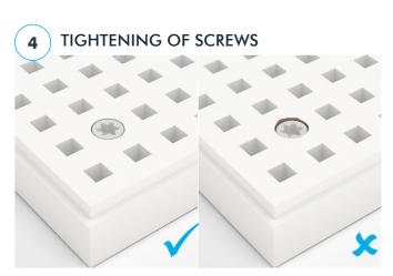
• IMPORTANT – the head of the screw must be levelled with the surface of the panel. We recommend using a cordless screw-driver and adjust the speed to LOW.
