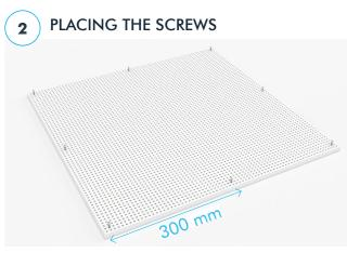
• Insert screws in 2<sup>nd</sup> perforation row (8 screws per panel).
