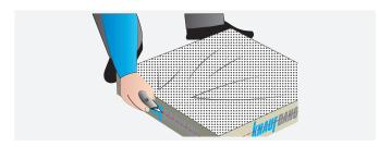
• Cut the plastic wrapping by running a knife along the sides of the package. Do not cut the plactic on top of the package.
