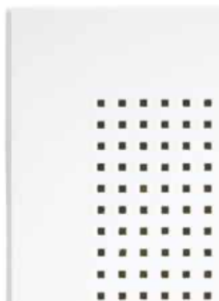
Micro, 3 x 3 mm, 8.3 mm c/c Perforation: 9.5-10.7%
