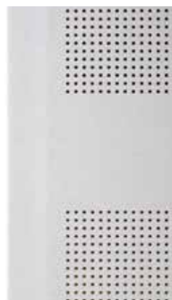
Micro, 3 x 3 mm, 8.3 mm c/c Perforation: 7.1 - 9.8%
