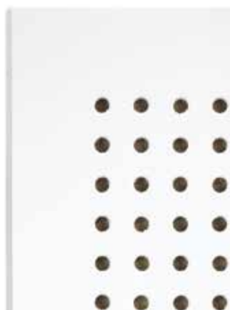
Globe, Ø6 mm, 15 mm c/c Perforation: 10.2%
