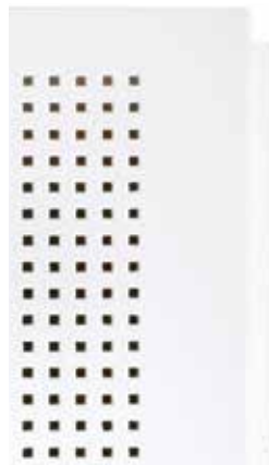
Micro, 3 x 3 mm 8.3 mm c/c Perforation: 9.9%
