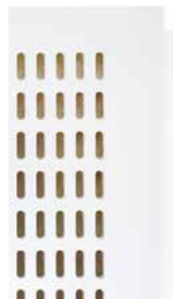
Tangent, 4 x 14 mm 10/20 mm c/c Perforation: 21.6%
