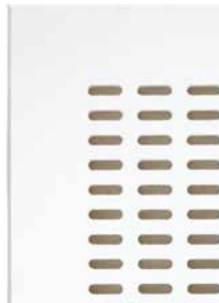
Tangent, 4 x 14 mm, 10/20 mm c/c Perforation: 21.1-21.3%
